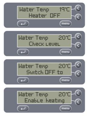
To continue using the Grant digital ultrasonic bath, refill with liquid up to the liquid level sensor and switch the unit off and on again.
